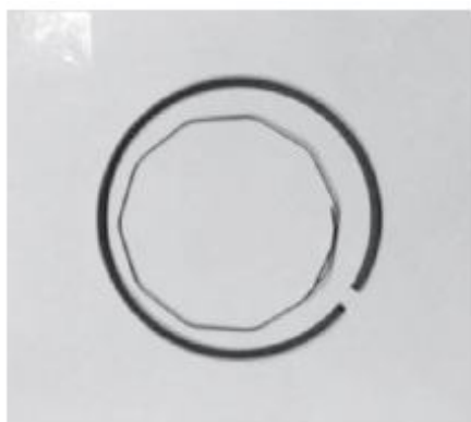
Figure 3.4: Piston rings for a two-stroke engine. The expander put at the center takes free state. When set into the piston ring groove, it spreads and gives additional force from the back of the second ring.
